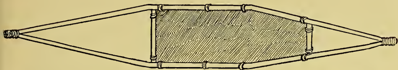
Fig. 295.—Bind the edges of the kago with grass or straw like this to make the frame.
